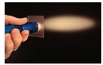
Figure 4 – Asymmetric diffuser
